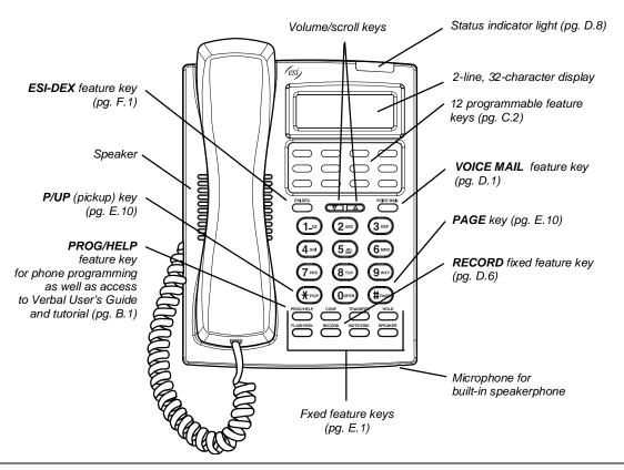
**Hint:** You can perform **direct programming** by holding down a programmable feature key for at least two seconds (similar to how you might program a car radio button). This isn't applicable to the fixed-feature keys which, as their name implies, are already programmed.
