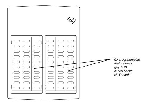
**Hint:** You can perform **direct programming** by holding down a programmable feature key for at least two seconds (similar to how you might program a car radio button). This isn't applicable to the fixed-feature keys which, as their name implies, are already programmed.
